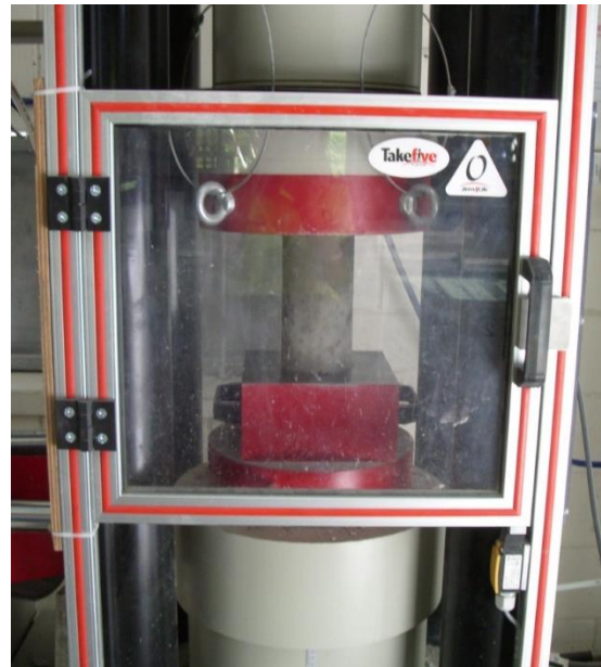
Figure 26.10 – Test in Compression Machine
