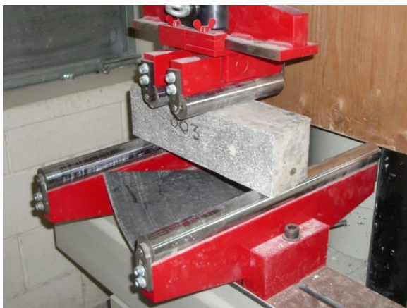
Figure 26.12 – Flexural Testing Beam in Test Rig
